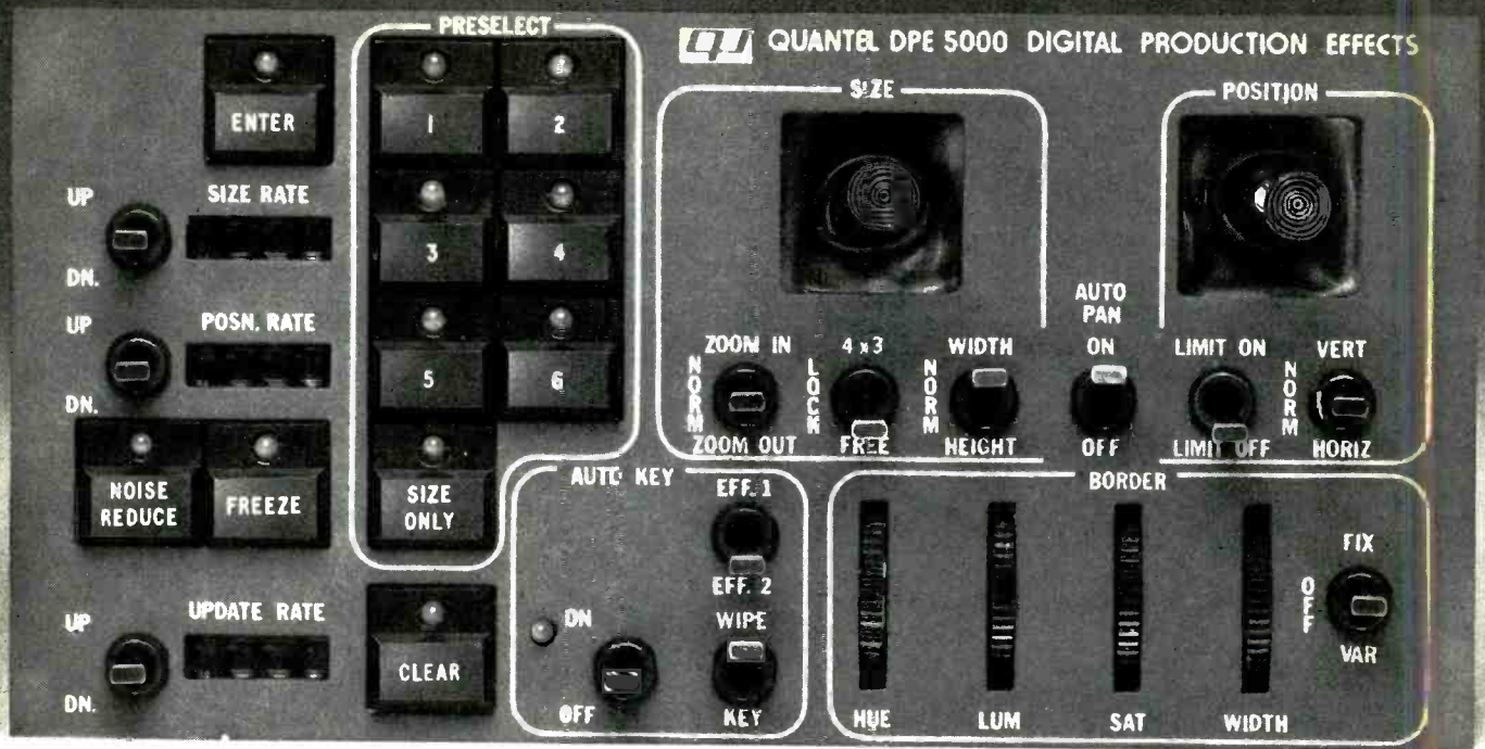
Production control panel of the DPE 5000.
